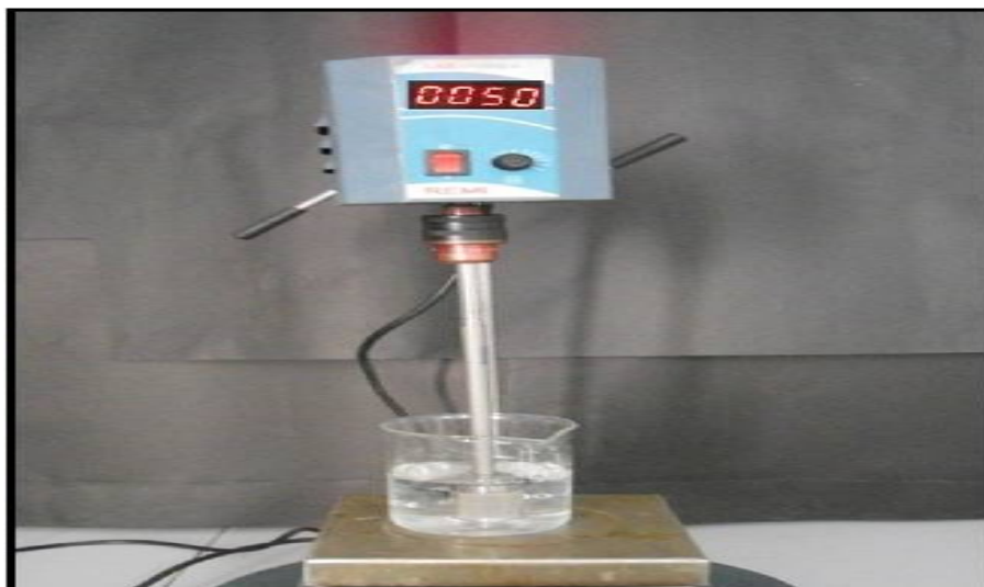
Figure 4. Modified in-vitro dissolution test apparatus (basket type).
